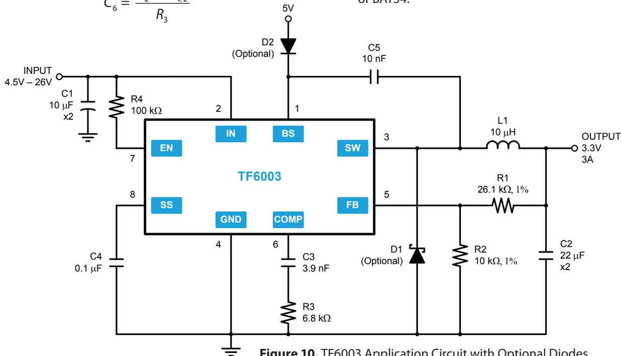
Figure 10. TF6003 Application Circuit with Optional Diodes
