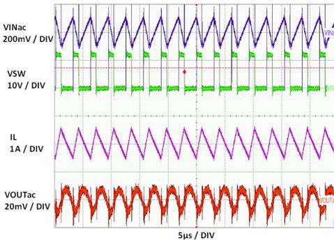
Figure 3. 3A-Load Steady State Operation
