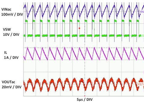
Figure 2. 1.5A-Load Steady State Operation
