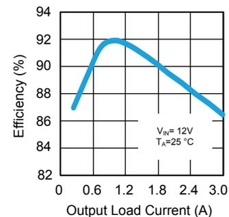
Figure 8. Efficiency as a Function of Load
