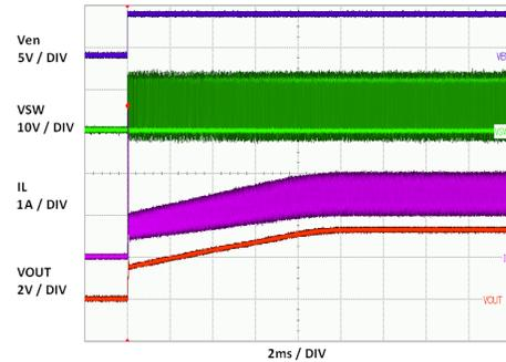
Figure 5. 1.5A-Resistive-Load Startup Via Enable Operation
