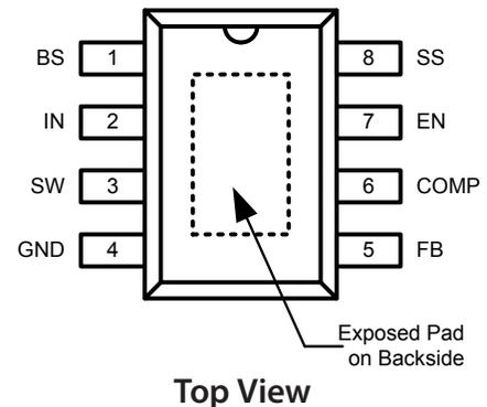
**3A, 26V Synchronous Rectified Step-Down Converter**
