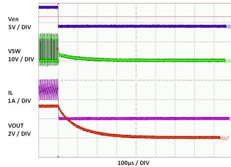
Figure 6. 1.5A-Resistive-Load Shutdown Via Enable Operation
