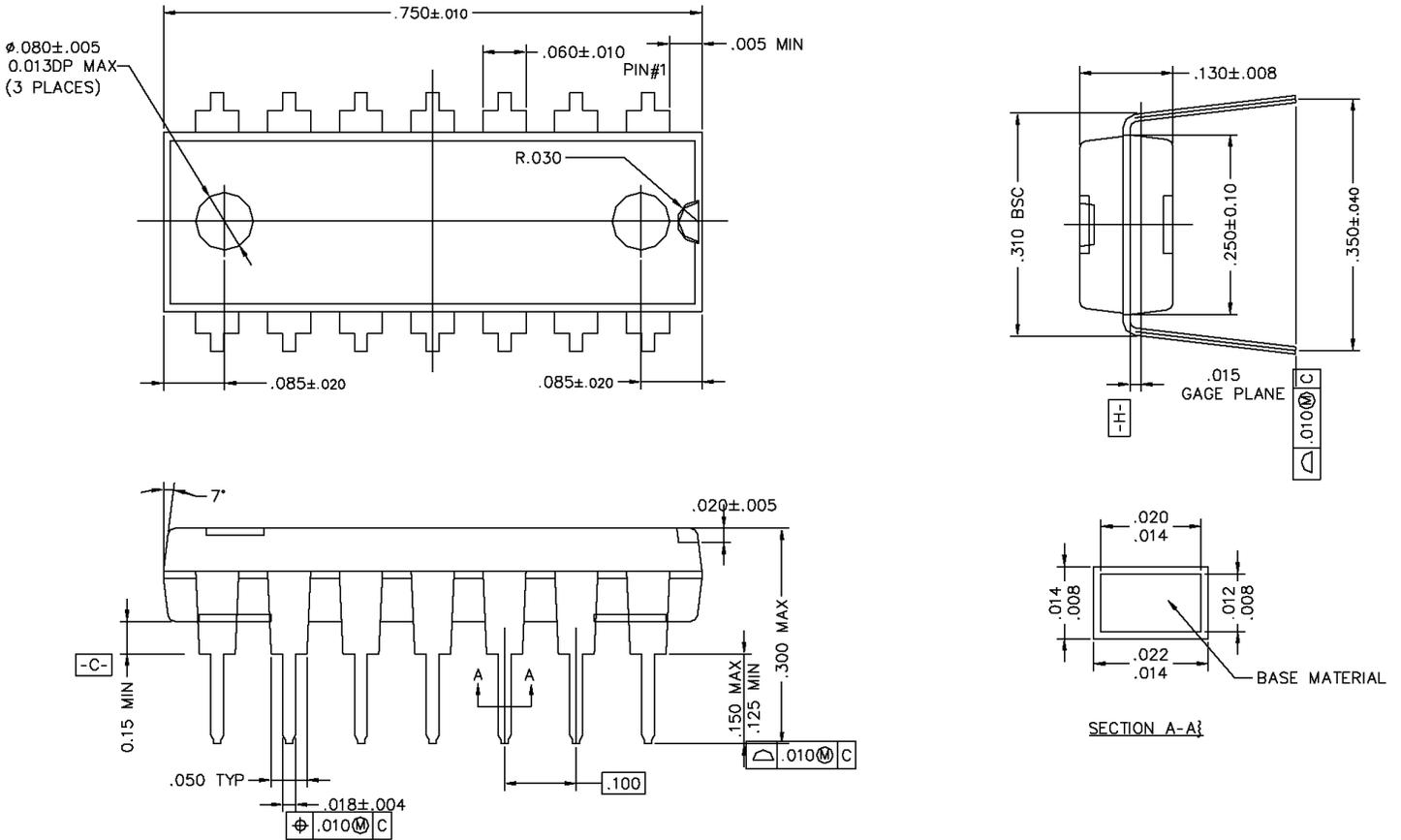
Note: Drawing conforms to jedec ref. MS-001 rev D
